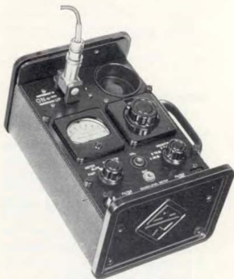
Figure 1. View of the Sound-Level Meter with microphone replaced by connector.
